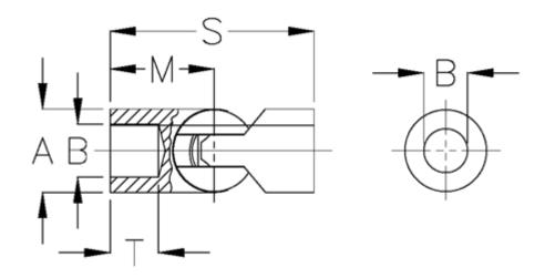
$\begin{array}{lll} A & = 40 \\ B \ H7 & = 20 \\ M & = 50.0 \\ Max \ torque \ (Nm) = 160 \\ s & = 100 \\ T & = 24 \end{array}$
